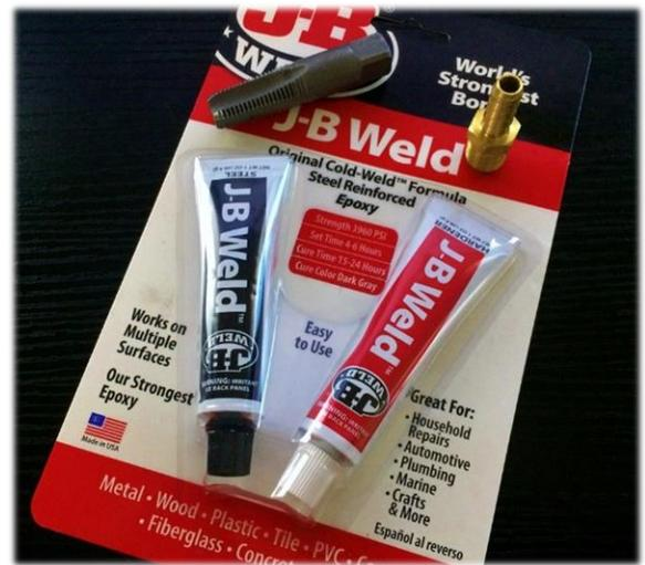
**Figure 3: Parts needed for tapping the stock manifold. I used Vermont America 20372 1/4” to 18 NPT tap, and Parker 4-4 B2HF-SS fitting (SS version; brass is shown above).**
