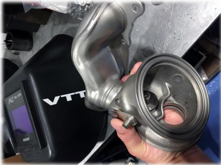
Figure 1: VTT OEM/Stage 1 manifold/housing with internal wastegate
