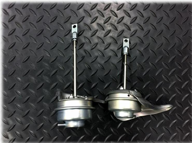
Figure 3: Wastegate actuators; different lengths for different applications
